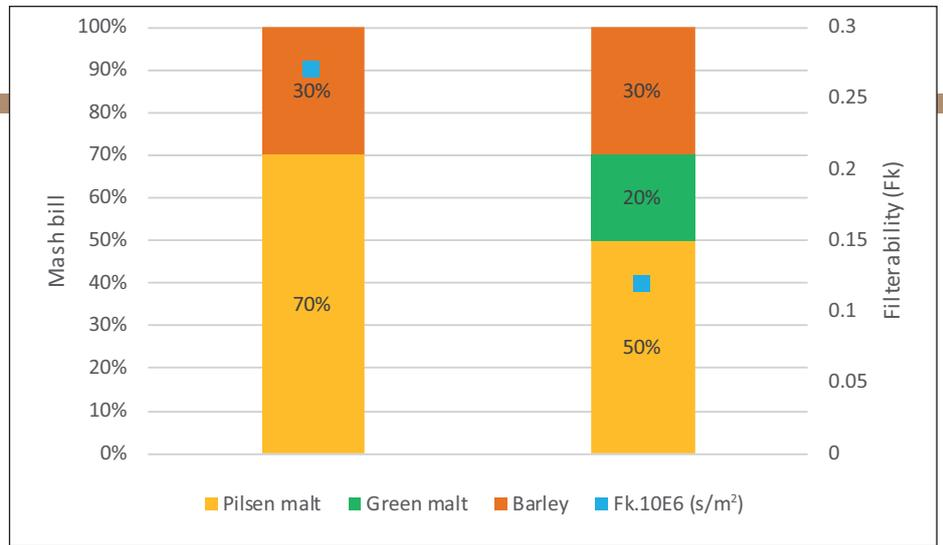
**Fig. 3 Green malt improves filterability (Fk is inversely correlated with filterability)**
